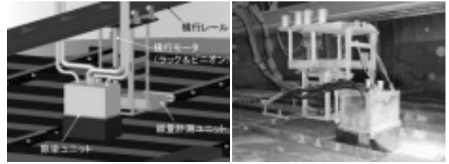
Fig. 6 Decontamination equipment for bottom
